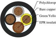
Polychloroprene rubber outer jacket Bare copper conductor Green/Yellow wire EPR insulation
